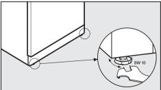
To align the appliance, adjust the feet using a suitable spanner.
