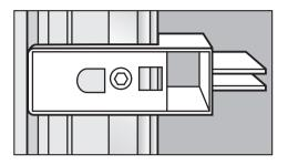
Do **not** remove the installation supports from the appliance door.
