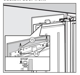
Open the door and hang the custom door with the mounting frame over the threaded bolts <sup>1</sup>/<sub>2</sub>.
