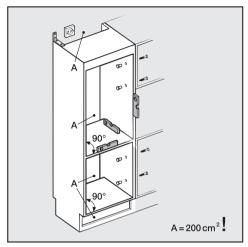
Before installing the appliance, the housing unit must be carefully aligned using a spirit level. The housing unit corners must be at right angles, as otherwise the appliance furniture door will not align correctly with the 4 corners of the unit.
