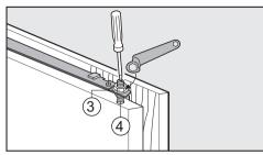
Whilst counterholding adjusting bolts
