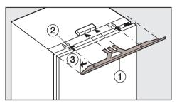
Slide cover strip ① into the holder as shown, with the bumps facing downwards. The bumps will fit into keyhole slots ②. The cover strip is then flush with the side of the appliance on which the door is opened ③.
