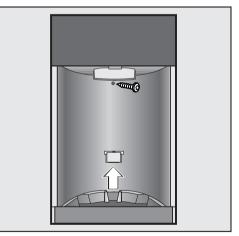
Remove the screw from the rear casing, then lift the tab on the drip tray up and off.
