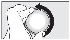
Turn the light cover counterclockwise and pull out.
