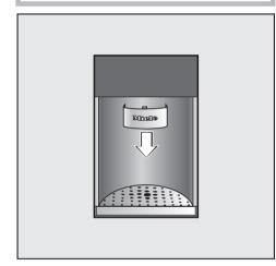
Press the dispenser back and pull downwards to remove.
