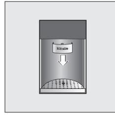
Press the dispenser back and pull downwards to remove.
