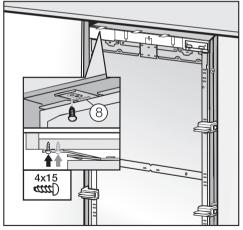
Screw the attachment plate lugs (a) to the overhead furniture/fixtures.
