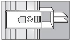
■ Do **not** remove the installation supports from the appliance door. They will be used later in the installation piche
