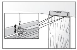
■ Tighten the nuts on the adjusting rail.
