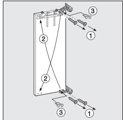
■ Unscrew and remove screws ①.
