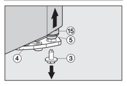
■ With the help of another person, carefully tilt the appliance backwards and pull hinge pin ③ out of the lower right hinge plate ④.
