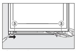
Slide the soft-close mechanism back into the door as far as it will go towards the appliance using a flat-headed screwdriver.
