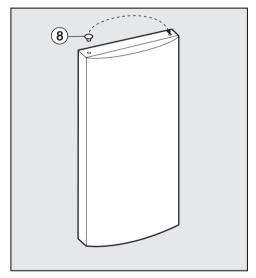
Remove cap ® from the hinge bush in the door and refit on the opposite side.
