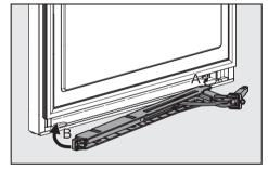
Insert the soft-close mechanism back into the door, starting at the right hand side.
