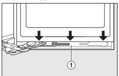
■ Gently remove panel ① from the soft-close mechanism by inserting a flat-bladed screwdriver into the gap from above and easing it off bit by bit.
