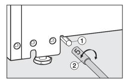
■ If necessary, also align the two rear adjusting devices ① using socket wrench ②.
