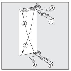
Remove screws ①, and use the stoppers supplied ③ to plug the empty holes.
