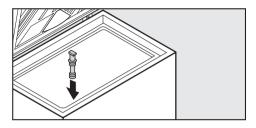
Use the stopper supplied to plug the defrosting outlet in the bottom of the interior of the appliance.
