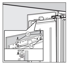
■ Open the door and hang the custom door with the mounting frame over the threaded bolts (1).
