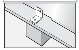
■ Loosen the bracket that holds the appliance to the pallet.
