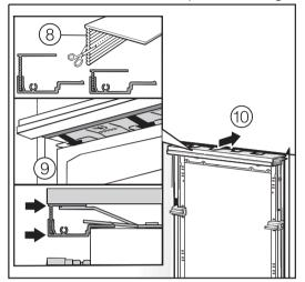
If there is a fairly large gap above the appliance, cut a wooden beam to fit exactly and place it in the gap.
