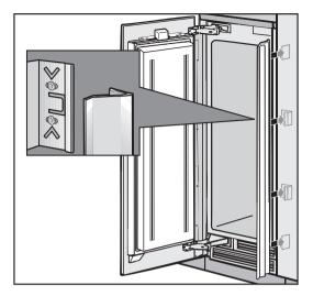
Insert the cover strip into the space between the appliance and the wooden panel.
