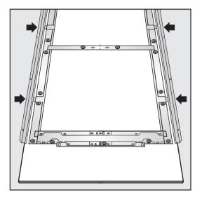
Insert the angle trim (3) as far as it will go in the spaces provided in the mounting frame.
