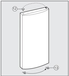
Remove cap (2) from the bearing bush in the door and refit on the opposite side.
