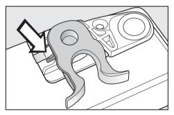
Using a screwdriver, remove spring clamp <sup>(1)</sup> from underneath the door and fit it on the opposite side.
