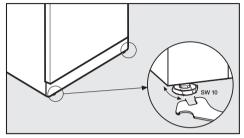
■ **Ensure** that you unscrew adjusting foot ① from the hinge plate until it sits on the floor. Then unscrew the foot by a further 90°.
