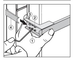
Loosely attach the handle to the opposite side of the door with the two front screws 2. Mounting plate ③ must be positioned on the side of the door so that when the door is **closed** it is flush with the side of the appliance.
