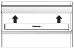
■ Pull the active charcoal filter holder upwards to remove it from the shelf.
