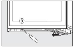
■ Attach the spacer and the soft-close mechanism securely using screw ③.
