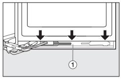
Prise open panel ① from the soft-close mechanism and ease it off carefully from above bit by bit. Take care not to damage the door seal.
