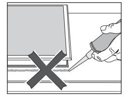
The sealing strip under the edge of the top part of the appliance provides a sufficient seal for the worktop.
