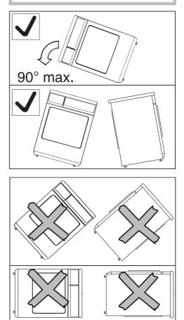
If the tumble dryer has not been transported as described, then it must be left to stand for at least 1 hour before it is connected to the electricity supply. Otherwise the heat pump can be damaged.
