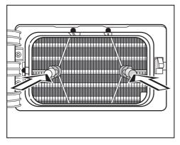
First insert the handle with the filter attached over the two guide pins.
