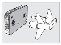
Fit the filter back on the handle. Make sure it is the correct way round.
