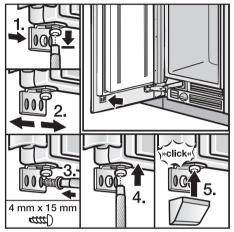
The fixing brackets are used to secure the custom door front to the bottom of the appliance door.
