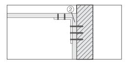
Two anti-tip brackets are recommended for each appliance. For side-by-side installations 4 brackets are recommended.
