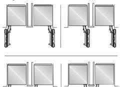
If there is a partition with a thickness from  ${}^5/{}_8$ " (16 mm) to 6  ${}^5/{}_{16}$ " (160 mm) between the adjacent appliances, then each appliance should be individually installed within its own niche using the mounting accessories included. The "Merging Kit" will also be needed.
