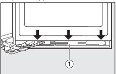
■ Remove panel ① from the soft-close mechanism by inserting a flat-bladed screwdriver into the gap from above and easing it off bit by bit.
