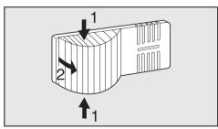
Press the sides of the lamp cover inwards (1), disengage the cover (2) and unclip it at the rear. Replace the lamp.
