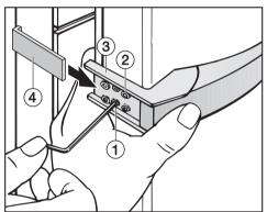
Loosely attach the handle to the opposite side of the door with the two front screws (2).
