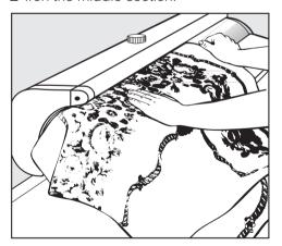
■ Fold in half with unironed edges together and place over the left end of the roller with the ironed middle section hanging over the edge to prevent creasing. Then pass both sides of the the non ironed sections through the rotary iron.
