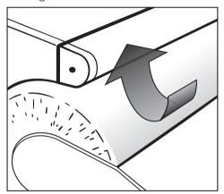
If you lift the finger guard now, the roller stops rotating and the heater plate rises.
