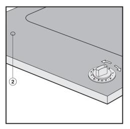
The Operating indicator light / Residual heat indicator ② will illuminate when the control knob is turned on. As long as the burner is hot, this light will remain on. Once the surface temperature has reached a safe level, the light will go out.
