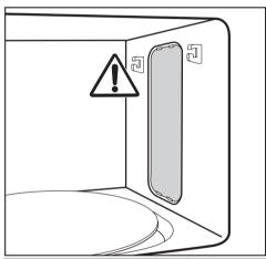
Do not remove the cover to the microwave outlet inside the oven.
