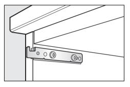
To secure the spacers and hooks, place a screw in one of the front two holes and another in the middle of the long hole at the back.
