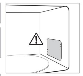
Do not remove the cover to the microwave outlet inside the oven, nor the film covering the inside of the door.
