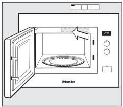
Stick the enclosed short instructions to the frame behind the door as illustrated, making sure they do not block any of the vents. For safety reasons, this appliance may only be used when it has been built in.
