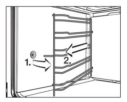
Pull the runners forwards out of the holder and remove. If applicable, also remove the catalytic side panels attached to the runners.
