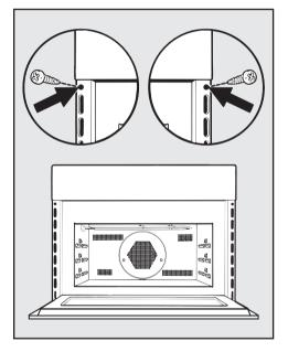
Open the oven and fix the appliance with the two supplied screws at the side panels of the cabinet.
