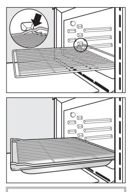
When inserting a rack, always check that the safety notches are at the rear of the oven.
