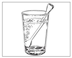
When heating liquids, milk, sauces etc. in the microwave without the boiling rod, the boiling point of the liquid may be reached without the production of typical bubbles. The liquid does not boil evenly throughout. This so-called 'boiling delay' can cause a sudden build-up of bubbles when the container is removed from the microwave or shaken, which can lead to the liquid boiling over suddenly and explosively. Danger of burning.
