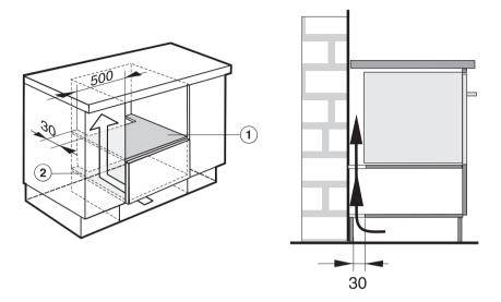
To ensure sufficient ventilation to the oven, a cut-out of 500 x 30 mm is required in the base of the building-in recess (1) and in the bottom of the housing unit (2). The furniture housing unit must not have a back panel fitted behind the building-in niche.
