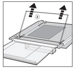
The individual glass panels can now be cleaned with a sponge and a solution of hot water and a little washing-up liquid. Dry thoroughly with a soft cloth.
