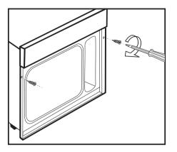
Secure the appliance by screwing the two wood screws
