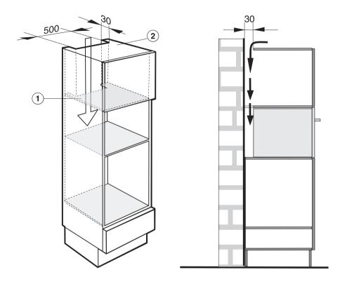
To ensure sufficient ventilation to the oven, a cut-out of 500 x 30 mm is required in the interim shelf above the building-in recess ① and in the top of the housing unit ②. The furniture housing unit must not have a back panel fitted behind the building-in niche.
