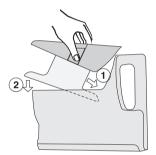
After cleaning, dry both parts of the insert thoroughly before replacing it in the water container. When replacing the insert, guide it in at an angle ① and then push it downwards ② as illustrated.
