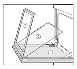
In the rare event that condensate or soiling has worked its way in between the glass panels, the door can be dismantled in order to clean the individual panels.
