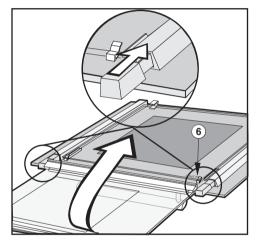
Then push the inner panel a back into its retainer until it clicks into position (see detail).
