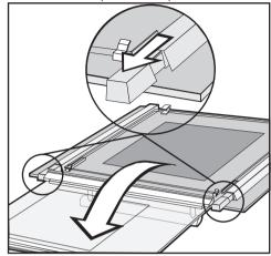
Push the middle glass panel ② in its retainer ④ in the direction of the arrow into the front clips ⑤.
