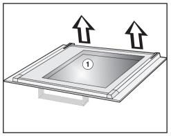
Open the inner panel towards you. Then pull it out as far as possible in its retainer (see detail).
