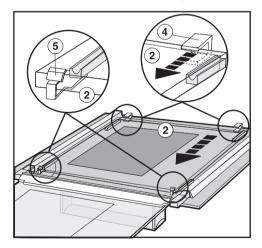
Pull the middle panel ② upwards out of its retainer at the back and then remove it from the front clips.
