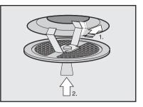
■ Hold the ceiling filter at a slight angle to insert it.
