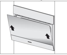
Do not lift the door at the door handle. The handle and door panels could be damaged. Make sure that the door is not tilted during removal.
