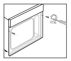
Secure the appliance to the left and right side of the cabinet with the two supplied 1/8" x 1" (3.5 x 25 mm) wood screws. ACAUTION: Before installation or servicing, disconnect the power supply by either removing the fuse, shutting off the main power or manually "tripping" the circuit breaker.
