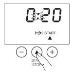
"Start" will appear in the time display, the → symbol will stop flashing, and the colon will begin to flash.
