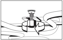
Unscrew the locking nut from the element to release it.
