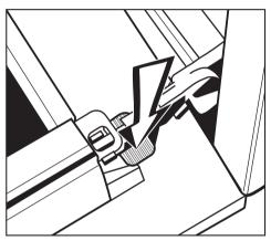
Push down the locking clamps on each door hinge.
