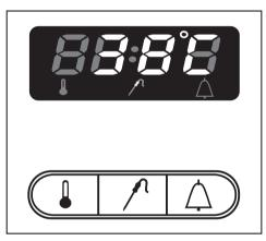
the actual core temperature appears in the oven display. N.B. The lowest temperature that can be displayed is 20°C, so this will also be shown until the roast probe registers 20°C.
