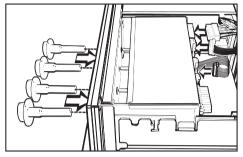
Insert the hob control knobs into the control facia.
