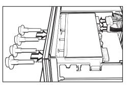
Insert the hob control knobs into the control facia.
