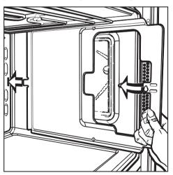
■ Ease the back lug into the opening in the rear wall.
