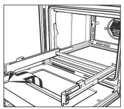
■ Remove the frame from the guide rails.
