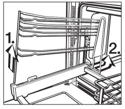
■ Pull out the telescopic carriage and remove the side runners.
