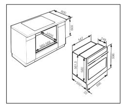
■ Push the cooker into the housing unit as far as the oven trim and align.
