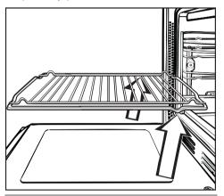
When pushing the tray, pan and rack back in, always ensure that the safety notches are at the rear of the oven. (See illustration)
