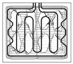
For grilling large quantities of thin cuts and for browning food in large dishes. The whole of the grill element is switched on.
