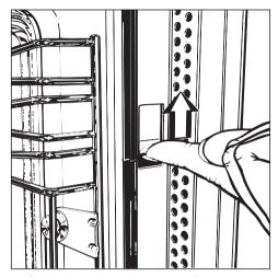
Slide the relevant access flap upwards.
