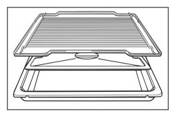
To be placed in the grill pan / oven tray when grilling and roasting.
