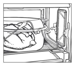
When roasting poultry, the best place to insert the probe is the thickest part between thigh and body.
