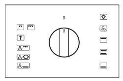
The function selector can be turned clockwise or anti-clockwise.
