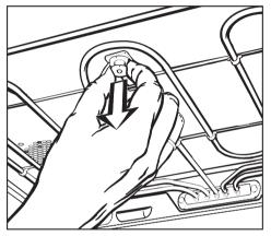
Pull down on the fixing knob for the element to release it.
