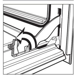
Flip up the locking clamps on each door hinge. This locks the hinges.
