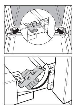
Slowly shut the door until the protruding clamps stop the movement. Pull the door upward. See illustration.
