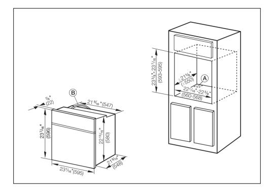
A Cut-out for power cord (min. 4<sup>"2</sup> / 10 cm<sup>2</sup>)
