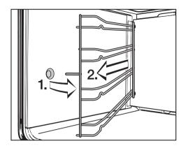
Reassemble in the reverse order, ensuring all parts are correctly in place.
