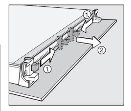
Push the spacers towards the centre of the door and then pull them off. If they are difficult to remove lift the middle pane up a little. The spacers should then be easier to move.
