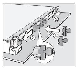
■ Lift the upper of the two middle panes up a little and refit the spacers to the panes. Then re-position them back next to the hinge guides.
