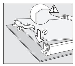
Replace the second of the middle panes. Make sure the cut-off corner is positioned at the top left hand side.
