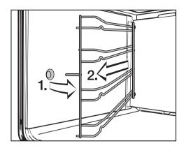
Remove the runners by pulling them out of the rear of the oven (2.)
