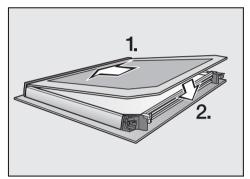
Push the inner pane into the plastic strip and place it in between the retainers.
