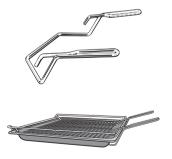
The handle makes it easier to take the universal tray, baking tray and rack out of the oven, or to put them into it. The two prongs at the top go inside the tray or above the rack, and the U-shaped supports underneath. Miele@home communication enabled appliances use the household electrical network ③ to communicate information about their operational status and the progress of the programme to a master appliance ④ / ⑤.
