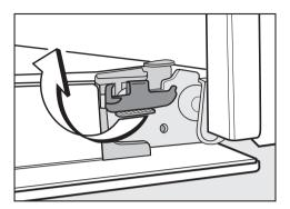
Flip both locking clamps back up as far as they will go into a horizontal position. Turn them as far as they will go into a horizontal position.
