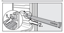
Fit the FlexiClip runner in between the two rails at the front (1) and then push it into the oven compartment (2).
