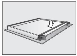
■ Refit the glass fibre seal.
