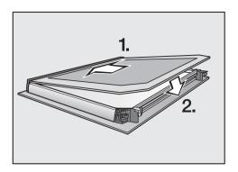
■ Push the inner pane into the plastic strip and insert it in the retainers.
