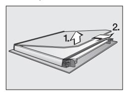
■ **Gently** lift the inner pane up and out of the cover strip.
