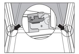
Before removing the door, the locking clamps on both hinges have to be released.
