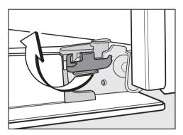
■ Flip both locking clamps back up as far as they will go into a horizontal position.
