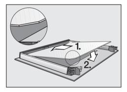
Replace the first of the middle panes. The more angled corner must be at the bottom left. When refitting the upper pane, the more angled corner must be inserted at the top left.
