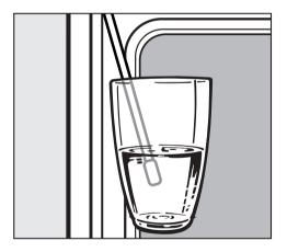
Hold a container with the quantity of water specified under the tube as shown. Start the water intake process with "OK". The amount of water required will be drawn up into the oven. As the water is taken in, bars will appear in the display. The amount of water specified will be more than the amount which is actually needed which means that some of the water will remain in the container as not all of it will be drawn up into the oven.
