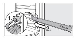
■ Fit the FlexiClip runner in between the two rails at the front (1) and then push it into the oven compartment (2).
