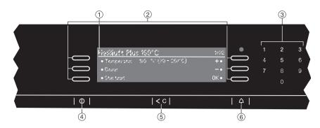
The appliance is operated via the display ① and the electronic sensors next to and below the display. These react to finger contact. A keypad tone will sound each time a sensor is touched. The volume of the keypad tone can be adjusted or switched off altogether (see "Settings - Volume - Keypad tone").
