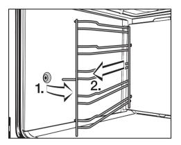
■ Pull the runners forwards out of the holder and remove.
