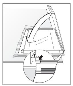
■ Hook the inner glass pane into the aluminium guides on the outer pane and lower it into position.
