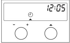
■ Whilst triangle ▲ is flashing, turn the (-/+) input dial clockwise until the required time shows in the display.
