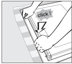
■ Finally using the ball of your hand press down on the aluminium trim on the inner pane to make sure it goes back into position. You will hear a very clear "click" when doing this. The retaining pins are pushed back out when you do this.
