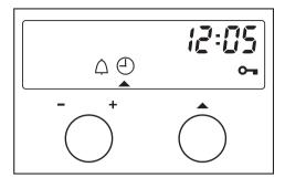
Use the **Function dial**, for selecting oven functions which require input e.g. the time of day.
