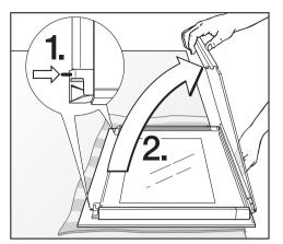
Press the pins near the hinge guides on both sides of the door in (1) to release the inner glass pane from its retainers.
