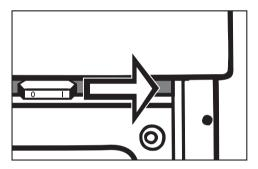
■ To switch the catalyser on, please push the lever located underneath the control panel to the right to position "I".
