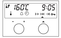
■ Call up the → symbol for duration by turning the function dial (right hand dial) until the triangle is underneath the middle arrow.
