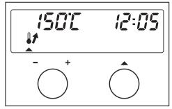
■ As soon as triangle starts to flash underneath the temperature symbol, use the (-/+) input dial to reduce the temperature to 150°.
