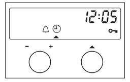
■ Turn the function selector (right hand dial) until triangle is underneath the symbol in the display.
