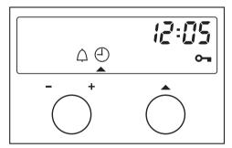
■ Turn the function selector (right hand dial) until triangle imes is underneath the ilde symbol in the display.
