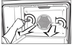
■ Loosen the screws in the back panel and remove.
