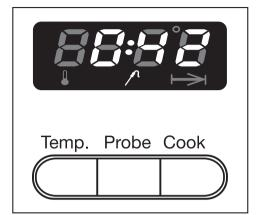
Once the oven has monitored the cooking process, it will calculate and display the remaining cooking time. The core temperature will no longer be displayed.
