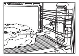
■ Insert the probe into the middle of the meat. Make sure that the probe does not touch any bones and is not located in a fatty area. Improper insertion of the probe could shut the oven off too early.
