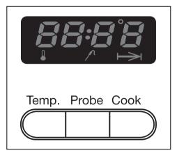
Each push button has a matching symbol in the oven display.
