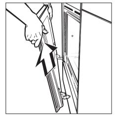
■ Lift up the door until the hinges disengage. Remove the door.
