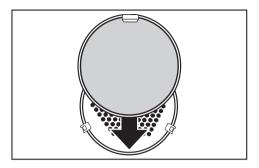
The filter helps to keep the oven fan clean from moisture and grease.
