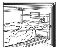
Insert the probe into the middle of the meat. Make sure that the probe does not touch any bones and is not located in a fatty area. Improper insertion of the probe could shut the oven off too early.
