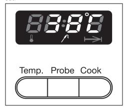
The **actual core temperature** will appear in the oven display. The lowest temperature that can be displayed is 67°F (20°C). This will not change until the temperature is greater than 67°F (20°C).
