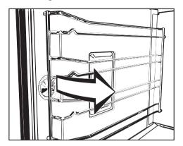
■ Pull on the fastener to release the runner.
