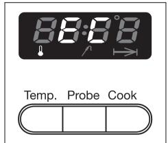
When using the "Cook" button or the roasting probe, the residual heat of the oven is automatically used to finish the cooking process and conserve energy.
