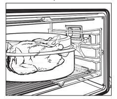
■ When roasting poultry, insert the probe into the thickest part of the bird between the thigh and body.
