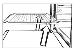
The racks have non-tip safety notches which prevent them from being pulled out completely while the oven is in use.
