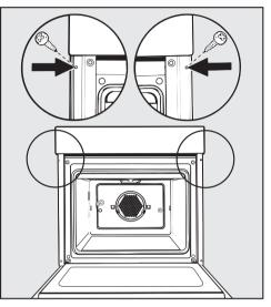
Open the oven door and locate the two mounting screw holes in the oven frame. Mark and drill 6 mm pilot holes. Secure the oven to the cabinetry by inserting screws through the frame and into the cabinetry. Only operate the appliance after it has been installed into the cabinetry.
