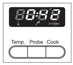
Once the oven has monitored the cooking process, it will calculate and display the remaining cooking time. The core temperature will no longer be displayed.
