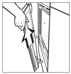
disengage. Remove the door.
