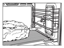
Insert the probe into the middle of the meat. Make sure that the probe does not touch any bones and is not located in a fatty area. Improper insertion of the probe could shut the oven off too early.
