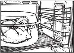
When roasting poultry, insert the probe in to the thickest part of the bird between the thigh and body.
