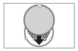
The filter helps to keep the oven fan clean from moisture and grease.
