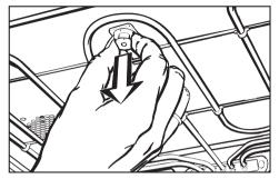
Pull and turn the fastener on the grill element to release it.
