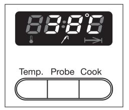
The **actual core temperature** will appear in the oven display. The lowest temperature that can be displayed is 67°F (20°C). This will not change until the temperature is greater than 67°F (20°C).
