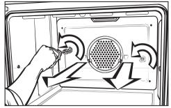
Loosen the screws in the back panel and remove.
