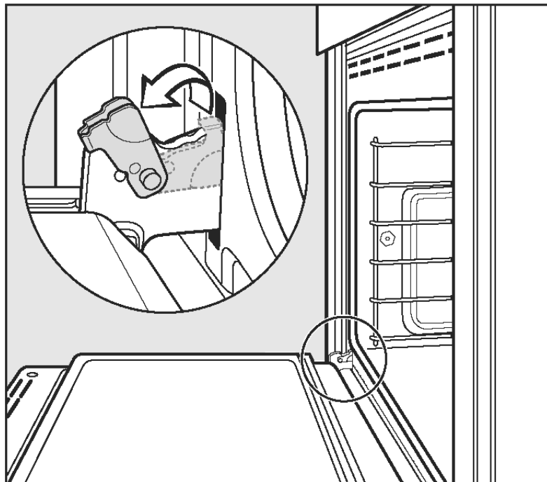
Figure 5-1: Door Hinge – Locking Tabs
