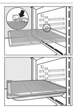
When inserting a rack, always check that the safety notches are at the rear of the oven.
