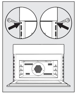
Open the oven and secure the appliance with the two supplied screws at the side panels of the cabinet.
