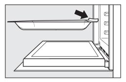
Always use the glass tray when using the Microwave (Solo) function.
