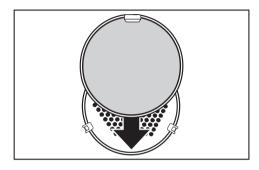
The droplets of fat caught up in the circulating air are deposited on the roasting filter. This helps to keep the oven and the area behind the interior back panel cleaner.
