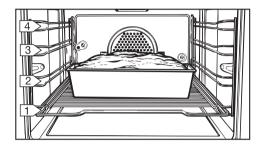
Place cakes in **rectangular tins** with the longer side across the width of the oven for optimum heat distribution and even results.
