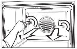
Loosen the screws in the back panel and take it out.
