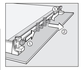
Push the spacers towards the centre of the door and then pull them off. If they are difficult to remove lift the middle panel up a little. The spacers should then be easier to move.
