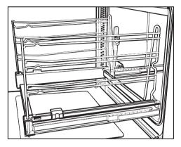
The telescopic baking carriage with 4 shelf levels can be drawn right out of the oven giving a good overview of cooking in progress.
