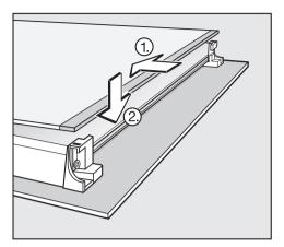
■ Finally replace the black printed inner pane. The print should face in towards the middle pane.
