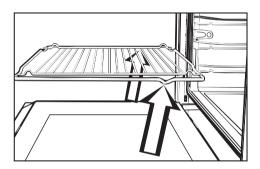
When pushing the tray, pan and rack back in, always ensure that the safety notches are at the rear of the oven (see illustration).
