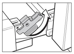
■ Slowly shut the door until the protruding clamps stop the movement. Pull the door upward. See illustration.
