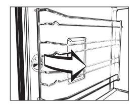
■ Remove the runners by pulling them out of the rear of the oven.
