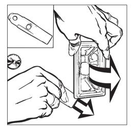
Press the lamp back into the sidewall of the oven and reinsert the cover.
