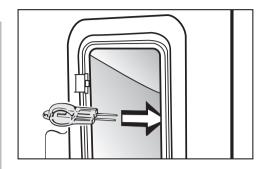
■ Put the light cover back in place with the notch to the rear of the metal clamps.
